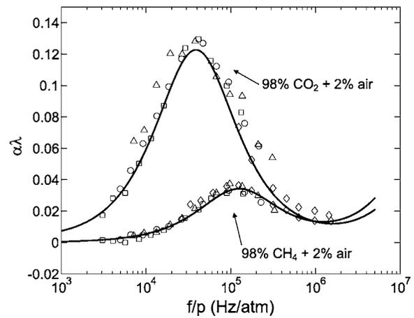
FIG. 4. Multiple-separation, four-frequency, test-cell measurements of the normalized attenuation for mixtures of  $CO_2$  and  $CH_4$  with air (symbols:  $\square$ , 92 kHz;  $\circ$ , 149 kHz;  $\triangle$ , 215 kHz;  $\diamond$ , 1 MHz). Curves represent the model predictions.
