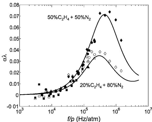
FIG. 3. Multiple-separation, multifrequency, test-cell measurements of the normalized attenuation for mixtures of 50% and 20% ethylene in nitrogen (symbols:  $\square$ , 92 kHz;  $\circ$ , 149 kHz;  $\triangle$ , 215 kHz;  $\diamond$ , 1 MHz; filled for 50% ethylene). Curves represent the model predictions.
